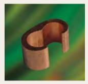
Copper "C"-Taps are range-taking compression connectors made from high conductivity copper alloy. They are used for making tap or parallel copper connections from 8 SOL to 4/0 STR conductors. C-Tap conectors provide consistent reliability with heavy wall construction that prevents relaxation of the joint after installation. Installation time is reduced because of its "C" shape. UL CU486A, 467 suitable for direct burial and CSA rated Electrical and Grounding.
