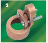
Threaded hub cast of high-strength, highly conductive bronze. Used with ground clamp to ground conductor to water pipe. Allows entry from any direction.
