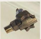
Transformer ground clamp bodies are cast from high conductivity, high strength copper alloy with cast high strength bronze eyebolts. Stainless steel nuts and lockwashers are standard on all clamps. For silicon bronze hardware, suffix catalog number with "-SB. The HTGE provides a hex or square shoulder for wrench tightening. The flat surface also acts as a seal to the tank. The TGE may be tightened by using a wrench on the body.
