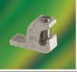
Lay-in lugs are used for grounding or in continuous loop bonding and are available in several variations, depending on the application. GLC-4 has a copper body with a steel screw and is used for general grounding applications with copper wire. GLC-4 DB and GLC-4 DBP have copper bodies with stainless steel screws and are UL Listed for direct burial in earth or concrete with copper wire.
