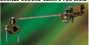
For connecting the grounding conductor in rigid conduit to water pipe. The copper strap allows flexibility during grounding and helps protect the conduit system from the results of vibrations in the water system. Assembled with zinc-plated steel screws.
