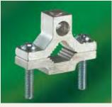
Dual-rated ground clamp that grounds aluminum or copper to water pipe, galvanized pipe or steel conduit. They are constructed from high-strength, extruded aluminum alloy and are plated to provide low-contact resistance.
