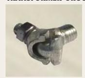
Transformer ground clamp bodies are cast from high conductivity, high strength copper alloy with cast high strength bronze eyebolts. Stainless steel nuts and lockwashers are standard on all clamps. For silicon bronze hardware, suffix catalog number with "-SB. The HTGE provides a hex or square shoulder for wrench tightening. The flat surface also acts as a seal to the tank. The TGE may be tightened by using a wrench on the body.
