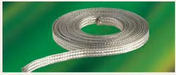
Woven of high conductivity, annealed, tinned copper wire, this braided ground strap provides maximum flexibility and ease of handling when installing ground or shield continuity. This braid is used for shield and lead-sheath grounding and is easily soldered to lead, copper and tinned metals. It is also used for continuing the fault-carrying capacity of the cable shield as a jumper braid.
