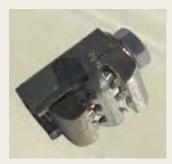
This clamp is specifically designed for use on self-supporting rural, figure 8 or IM type telephone cable when connecting the messenger to the ground wire. As the clamp is tightened it's insulation piercing teeth puncture the insulation of the messenger, eliminating the need for wire stripping and forms a positive ground connection. The bolt is made of stainless steel.
